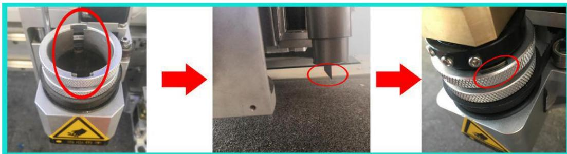
(3) Fix the black slot to the iron rod in the figure and insert the tool motor cable into the left socket.
