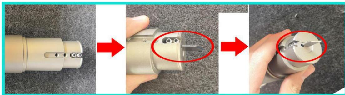
(2) The cutting edge of the knife must face the direction which the X-axis goes back to origin, tighten the circle ring.
