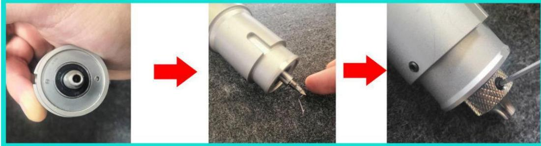
(2) The side of cutter edge must face the direction which the X-axis returns point, tighten the circle ring. The position of the black knob above the knife rod should be adjusted according to the cutting effect. If the material needs to be cut through, the knob should be fully tightened.
