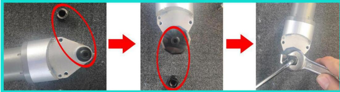
(2) After the cutter rod is placed in the cutter holder, tighten the circle ring and fix the slot to the iron rod at the figure. Tighten the screws at the connection between the tool rod and the tool head in the rightmost figure, and insert the motor cable of the tool rod into the left socket of the wires box.
