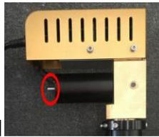
this position, until the tip of the knife drops to its lowest position. **B2.** Place a piece of typing paper on the table and drag the paper by hand. If the paper is just cut off, then the adjustment is done.
