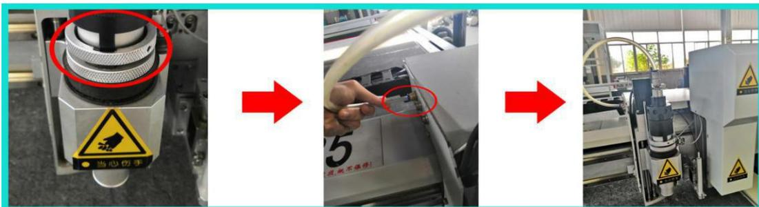
(3) Knife depth setting please refer to [6.1 Setting knife depth](#) → (4) [Judgment of the knife depth](#) → C, the air pressure should be adjusted to about 0.5mpa which according to the cutting material.
