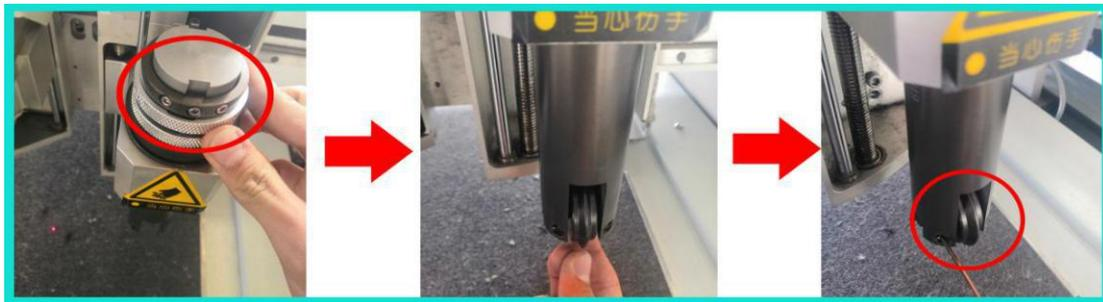
(3) When the creasing wheel is working, adjustment of the position of the creasing wheel dropping is the same as that of the knife depth setting, but the specific position is based on the actual folding effect ([Refer to 6.1 Knife depth setting and 6.1 knife depth setting \(8\)](#)).
