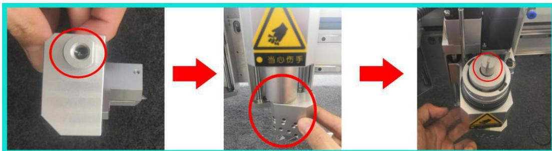
(4) Test and adjust the horizontal direction . A. Simply place the knife tip into
