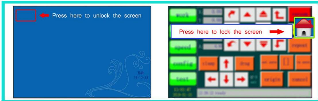
(Note: The screen saver interface is used to prevent the operator from accidentally touching the touch screen buttons, so there is no button in the screen saver interface. You can only press the upper left corner to wake up the screen and enter the work interface.)
